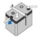
Disconnect the negative terminal first and avoid short-circuit caused by tools when removing old battery.
