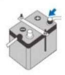
Connect the positive terminal first and check the terminal clamps for tight fit when installing new battery.
