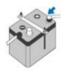
Connect the positive terminal first and check the terminal clamps for tight fit when installing new battery.
