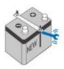
Clean corroded parts in tray and cable clamps before installation of new battery.
