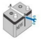
Clean corroded parts in tray and cable clamps before installation of new battery.
