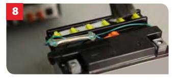
8. Wash spilled acid with water and baking soda solution, to ensure any acid is washed off the terminals.
