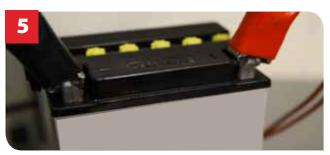
5. Prior to installation the battery should be completely charged for three to five hours at a current equivalent of 1/10 of its rated capacity as found in the specification pages of this guide. Eg. Use lamp charging current on a 10ah battery.
