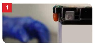
Remove sealing tube (red cap) and discard. Do NOT put this cap back on after the battery has been filled with electrolyte.
