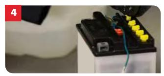
4. Loosely replace refilling plugs to avoid electrolyte spitting during charging.
