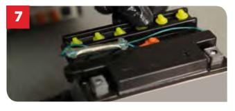
7. Check the filling plugs are securely fitted for screw in types – do not excessively tighten.
