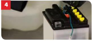
4. Loosely replace refilling plugs to avoid electrolyte spitting during charging.
