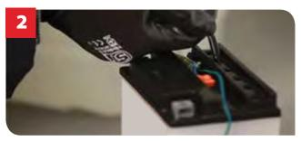
2. Remove filling plugs located on battery top. Fill with electrolyte to UPPER FILL level. NEVER use water or any other liquid to activate.
