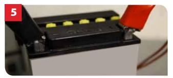
5. Prior to installation the battery should be completely charged for three to five hours at a current equivalent of 1/10 of its rated capacity as found in the specification pages of this guide. Eg. Use 1amp charging current on a 10ah battery.
