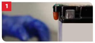
1. Remove sealing tube (red cap) and discard. Do NOT put this cap back on after the battery has been filled with electrolyte.
