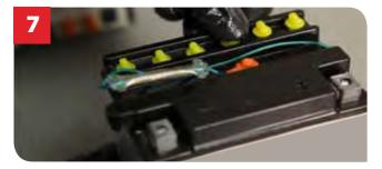
7. Check the filling plugs are securely fitted for screw in types – do not excessively tighten.
